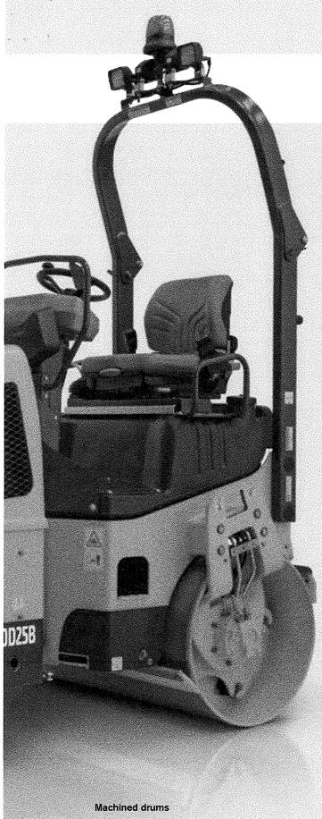
Machined drums with chamfered edges are perfectly round in order to produce a smooth, mark-free mat.
