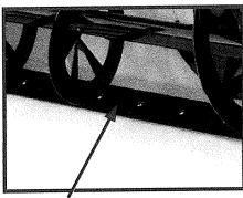
High grade steel bolt in replaceable cutting blade is standard and gives many years of trouble free cutting performance.
