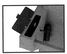
Enclosed chain case with spring tension tightner for idler sprocket maintains constant tension on the auger drive chain & reduces chain wear and possible freeze ups.
