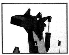
A double chute deflector with a standard 2" x 6" cylinder reduces blow back considerably in comparison to single deflectors.
